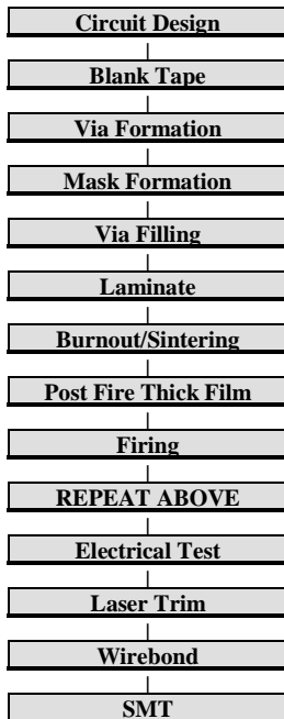
Figure 2: Basic Tape Transfer Process Flow
