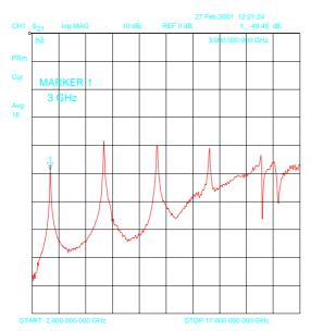
Figure 7: Dupont 943, Ag metallisation, 3GHz resonator
