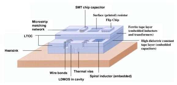
Figure 1: LTCC substrate with integrated passives
