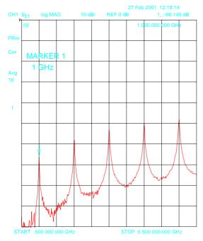
Figure 5: Dupont 943, Ag metallisation, 1GHz resonator
