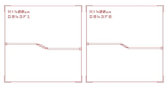
Figure 24: Layout of 28GHz and 42GHz coupled line filters
