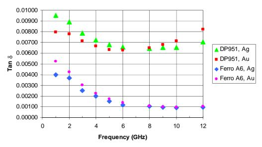
Figure 16: Measured loss tangent for Ferro A6 and Dupont 951 resonators, using Au and Ag resonators
