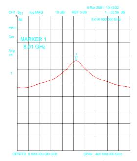
Figure 10: Close-in plot of the 2<sup>nd</sup> harmonic of the 4GHz resonator on Dupont 943, Ag
