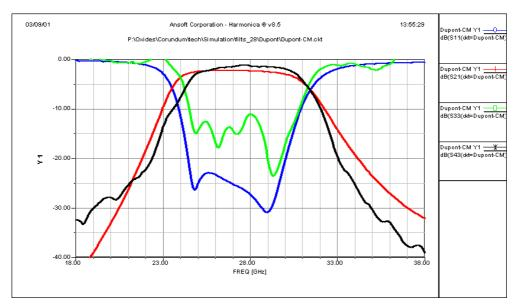
Figure 23: Measured versus simulated performance of mm-wave filter in Dupont 951, silver metallisation
