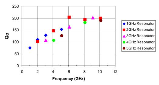
Figure 15: Unloaded Q of Ferro A6 resonators, Au metallisation
