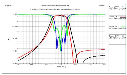
Figure 21: Comparison of measured to simulated performance of Dupont 943, 2.4GHz BPF, Au metallisation
