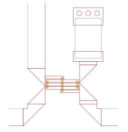
Figure 26: Close-in of layout detail of the 22GHz to 35GHz Lange coupler
