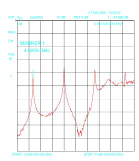
Figure 8: Dupont 943, Ag metallisation, 4GHz resonator
