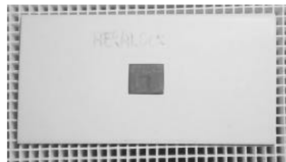
Figure 13: Co-fired ferrite transformer (top view)
