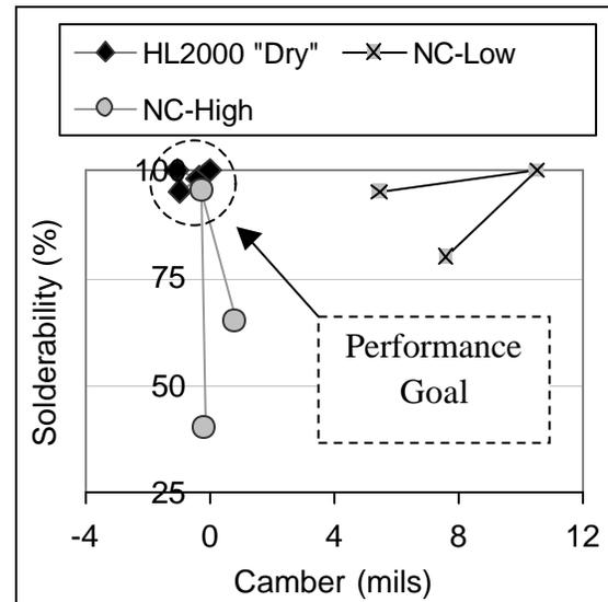
**Figure 13:** Scatter-plot of solderability versus camber for AgPd conductors printed on tapes with different amounts of free surface glass.
