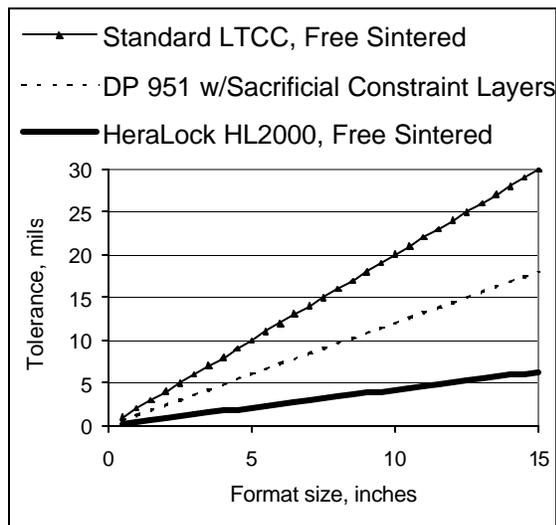
**Figure 4:** Positional tolerance plotted versus LTCC format size for three different processes.
