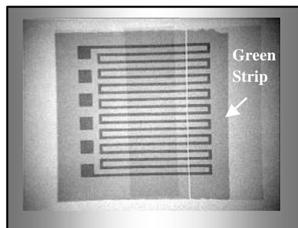
**Figure 3:** X-ray of test structure.
