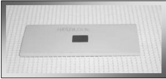
**Figure 7:** Ferrite transformer embedded in HL2000 before firing.
