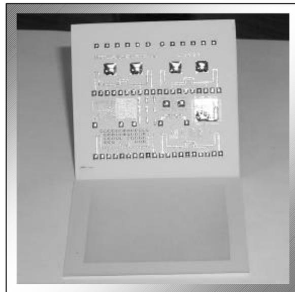
**Figure 14:** Samples of HL2000 modules. The top of part has been co-fired with AgPt conductor and dipped in 62-36-2 SnPbAg solder. The bottom part is a 100% coverage co-fired silver ground plane.
