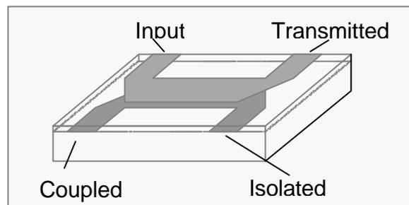
**Figure 1:** Broadside coupler. The structure requires precise alignment between two metal layers.
