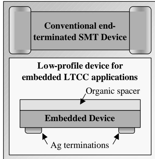
**Figure 10:** Proposed device configuration for embedded applications.
