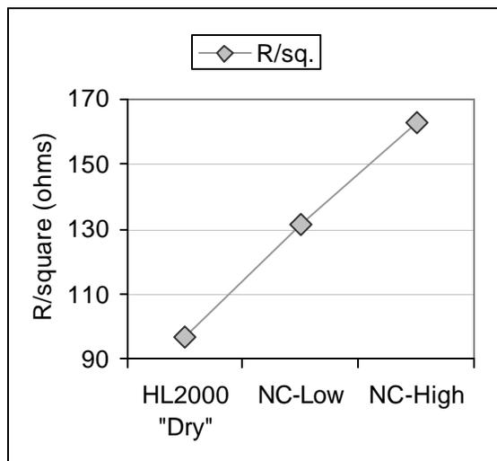
**Figure 12:** Resistance of a post-fired 100-  $\Omega$  paste @ 10  $\mu$  FFT on printed on tapes with different amounts of free surface glass.
