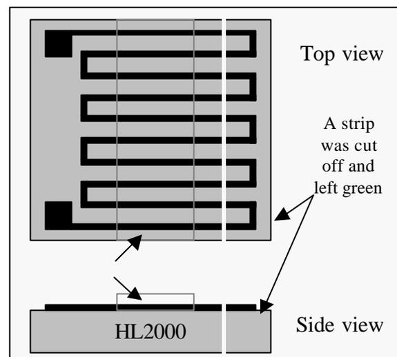
**Figure 2:** Test structure to evaluate surface and buried conductor shrinkage during firing.
