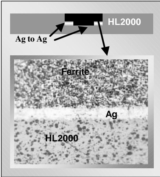
**Figure 8:** SEM micrograph of silver-silver contact of embedded ferrite structure.
