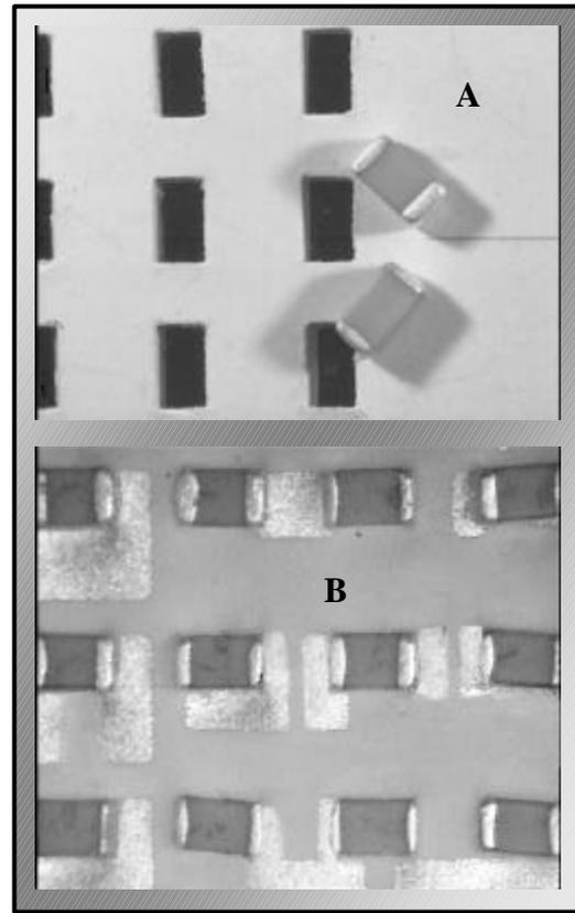
**Figure 9:** 0603 chip capacitors embedded in HL2000. A: Loose capacitors laying on HL2000 tape prior to lamination. B: Fired structure.
