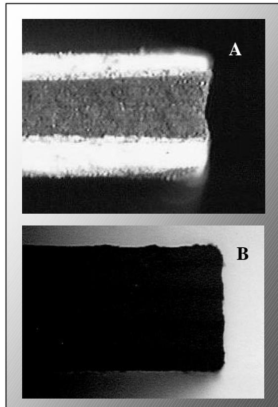
**Figure 6:** The walls of the surface-constrained LTCC (A) show necking due to the increasing shrinkage of layers further from the edges. In contrast, the walls of the HL2000 tape (B) remain nearly undistorted.
