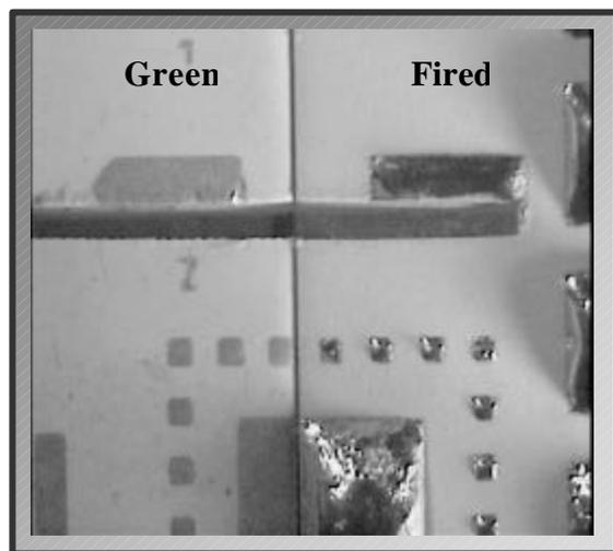
**Figure 5:** A slot cavity in HL2000. The part was cut before firing; the two halves were realigned after dipping the fired half in solder.
