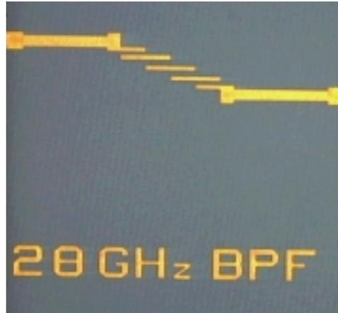
Figure 22: Photograph of one 28GHz BPF (overall tile width =15mm)
